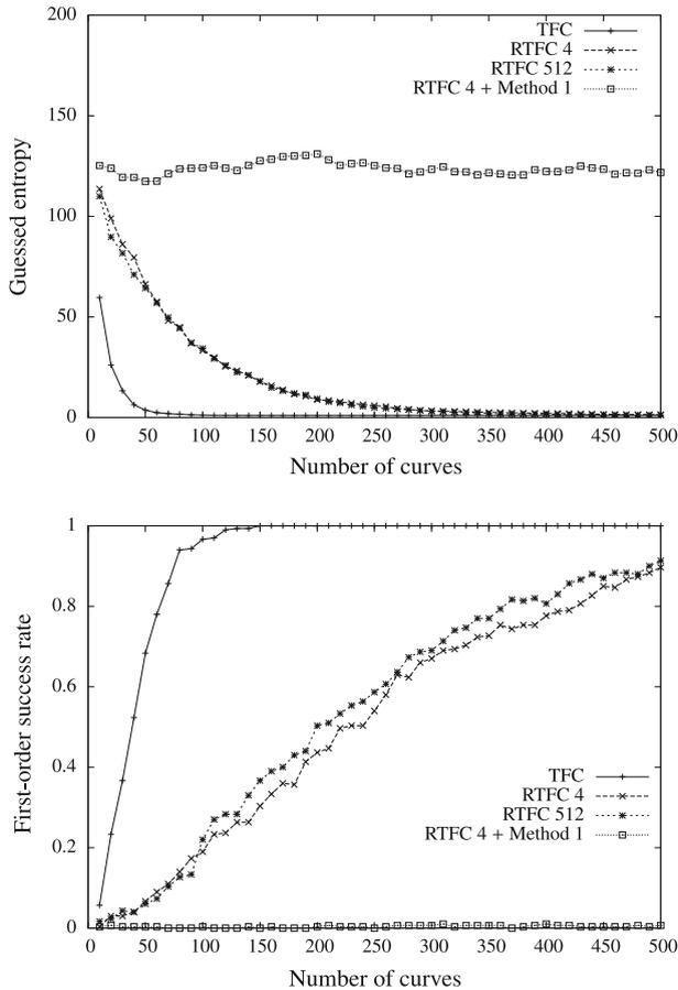
**Fig. 3** Side-channel attacks results using the guessed entropy and first-order success rate metrics from simulated curves. Comparison between AES implementations: basic using a TFC, using a randomized construction with 4 mappings (RTFC 4), using a randomized construction with 512 mappings (RTFC 512) and a randomized construction with 4 mappings combined with the masking method 1 (RTFC 4 + Method 1)
