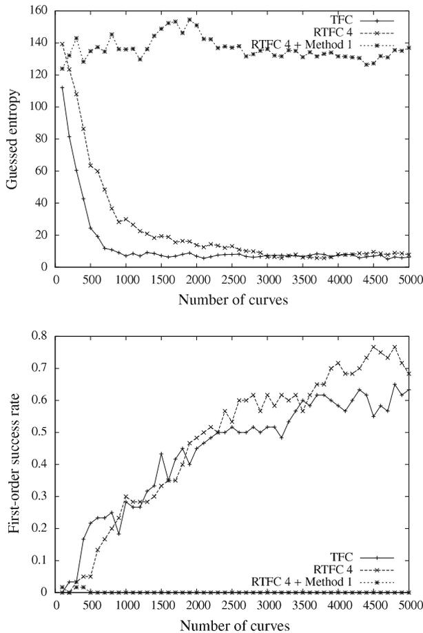
**Fig. 4** Side-channel attacks results using the guessed entropy and first-order success rate metrics from implementations on an AVR 8-bit ATmega 2561 processor. Comparison between AES implementations: basic using a TFC, using a randomized construction with four mappings (RTFC 4) and a randomized construction with four mappings combined with the masking method 1 (RTFC 4 + Method 1)
